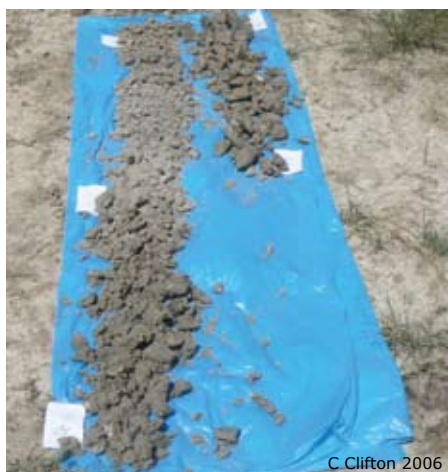
The soil (a Dermosol) was described to 1.5 metres and conductivity measurements were taken to measure salt content (refer to graph).
