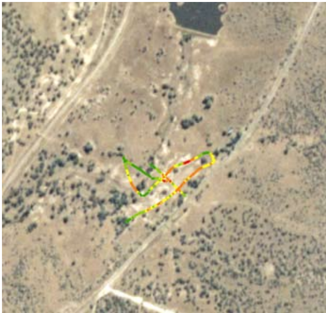
This figure shows areas with high salt levels (red parts of the lines) in the drainage line associated with scalding. The coincidence of bare ground with higher soils salinity levels suggests that there may be other areas of salinity nearby (e.g. below the dam, on the western side of the railway line).
